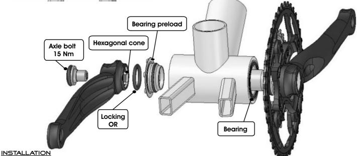
Check all parts very well cleaned, especially male/female of Hexagonal Cone, Axle bolt and thread.
