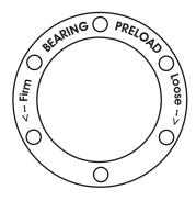
Shake crank-end to check BB play. Optimal tuning cancels axial play without adding any rolling resistance.
