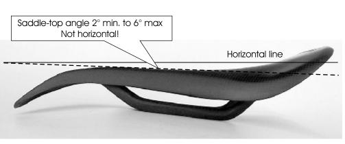
HyperSaddle's advanced ergonomy requires the fine adjustment of saddle-top anale. Adjust saddle-top angle as shown on figure (unllike conventinal saddles). Test ride several angle variations until you find find the optimal position for your body (change angle by small increments).
