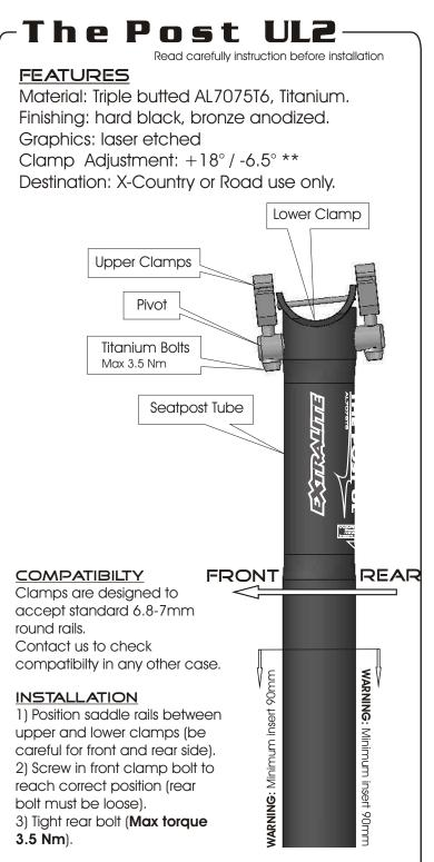
**Warning:** overtightening bolts may damage clamps and be very dangerous for your safety.
